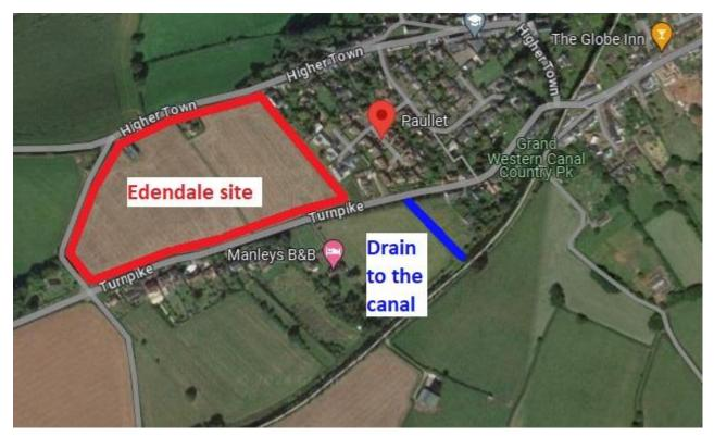
Given that the majority of the site has been bare soil all winter with lots of vehicles and foot traffic, creating and spreading mud, every time there is significant rainfall the drainage from the site reaches the Canal before silt is able to drop out of the water in the settlement pond.
